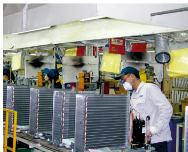
Outdoor units production
